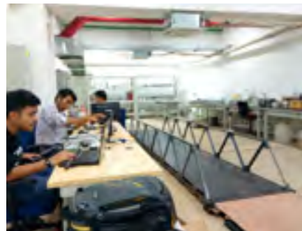
Testing bridge monitoring system in the lab © Pratama Budi Wijayanto
